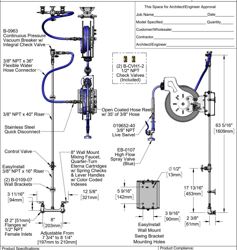
Open Coated Hose Reel w/ 35' of 3/8" Hose, High Flow Spray Valve w/ Swivel, Vacuum Breaker, 3/8" NPT Flexible Water Hose, 8" Wall Mount Mixing Faucet, 1/2" NPT Check Valves, Wall Brackets & Control Valve,
