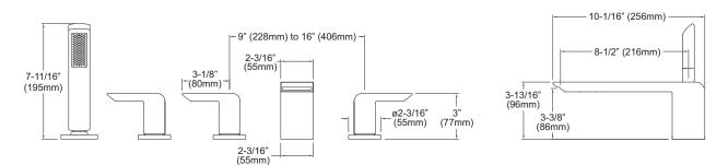
IMPORTANT NOTE: This valve/trim can only be installed in a built-up deck. It cannot be installed on pre-finished deck or on tub rim.
