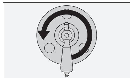
**Note:** Water Dance will run two functions simultaneously when the handle indicator is placed between two function emblems (totaling 6 functions).
