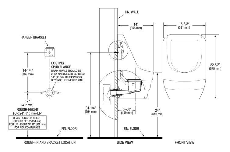
NOTE: ADA urinal rim height requirements allow all heights 17" and below. Sloan strongly recommends roughing in the drain to achieve a 16<sup>1</sup>/<sub>2</sub>" rim height or less to ensure compliance.
