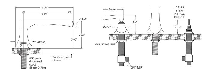
NOTE: Spout and valves install through 1-1/4" diameter holes.
