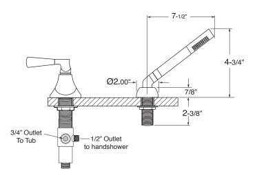
NOTE: 1/2" outlet for in-line vacuum breaker (18.15.055), and 60" chrome spiral hose (18.10.016) - INCLUDED
