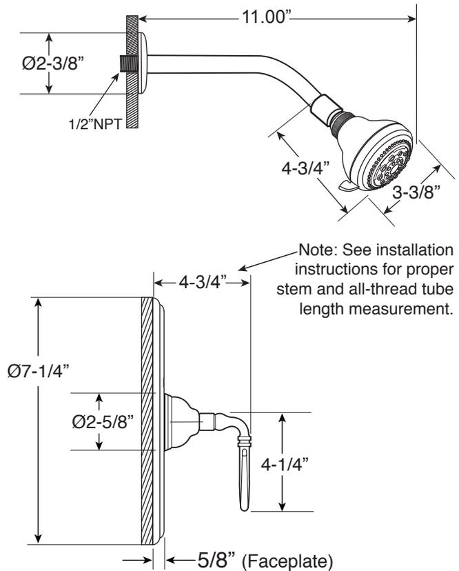
*Note: See installation instructions for proper stem and all-thread tube length measurement.*
