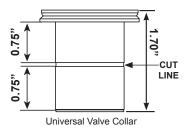
**Minimum Extension**: Minimum extension of 1" is achieved by cutting all three parts most severely.
