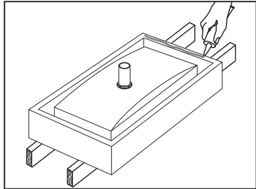
After checking fit and alignment, turn sink upside down and apply a generous portion of silicone adhesive around the under side of the rim near the edge. Place sink in position. Wipe off excess adhesive.
