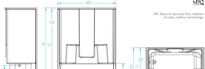
FEATURES Ibs Dimensional Tolerance ± %". Dimensions needed for site preparation should be measured from the unit. Aquatic assumes no responsibility for preparatory work.
