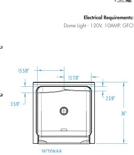
FEATURES lbs Dimensional Tolerance ± 3/8". Dimensions needed for site preparation should be measured from the unit. Aquatic assumes no responsibility for preparatory work.
