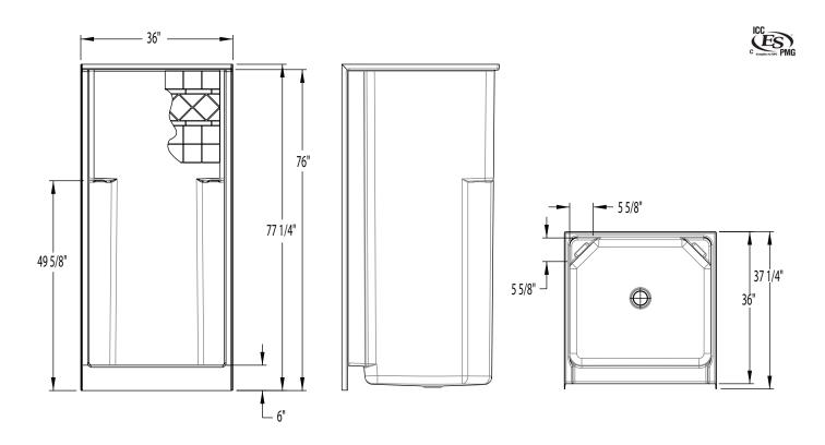
FEATURES Ibs Dimensional Tolerance ± %". Dimensions needed for site preparation should be measured from the unit. Aquatic assumes no responsibility for preparatory work.
